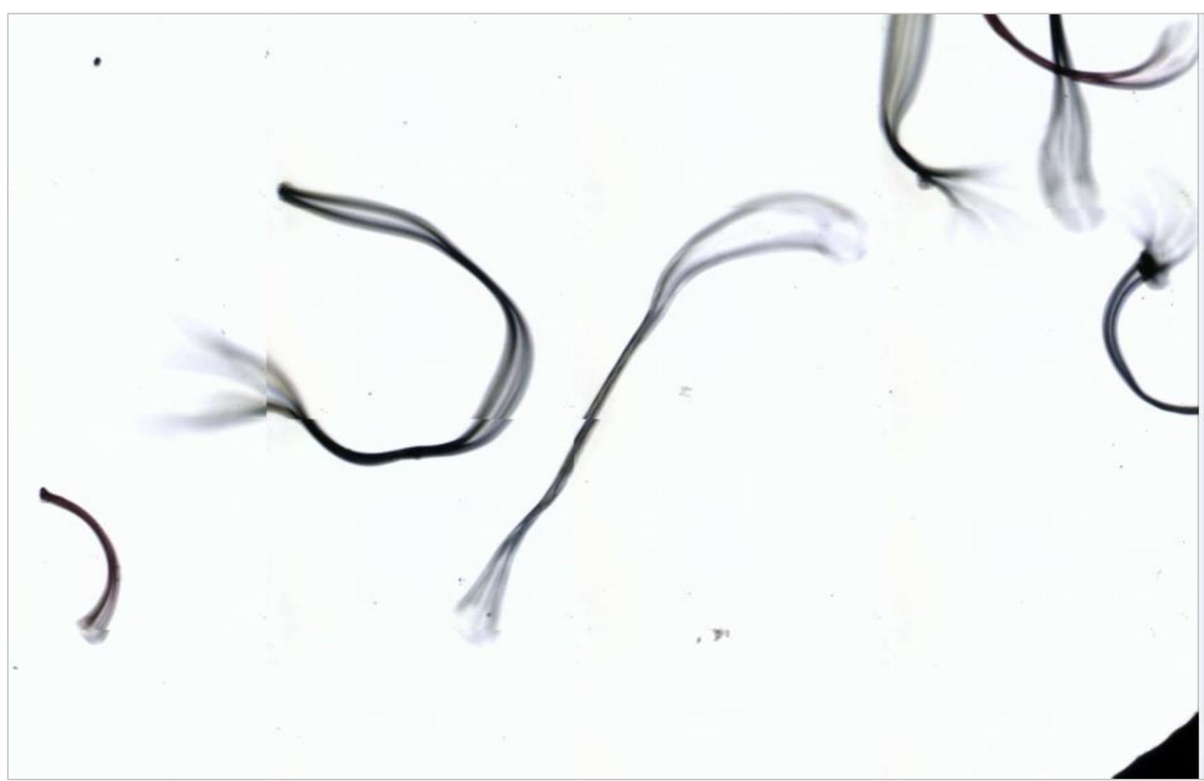
Figure 3: Polyester fibers found in laundry greywater
