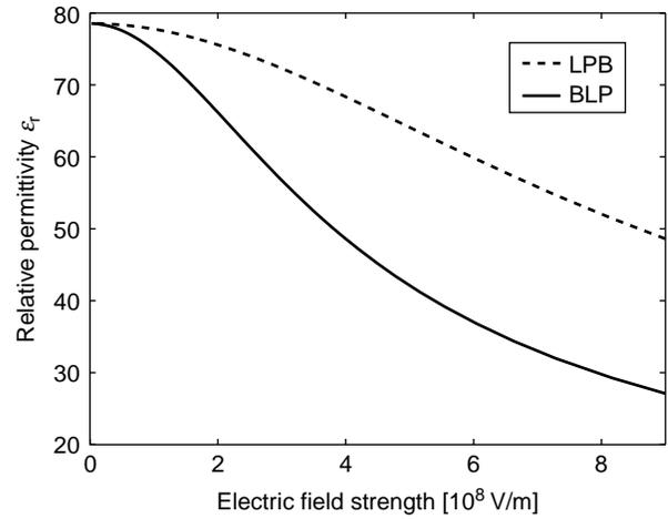
Figure 8. Relative permittivity  $\varepsilon_r$  as a function of the magnitude of electric field strength ( $E$ ) within the LPB model (Equation (69)) and BLP model (Equation (93)) for point-like ions and  $n_{0w}/N_A = 55$  mol/l, where  $N_A$  is the Avogadro number. In the case of the LPB model, the effective dipole moment of water  $p_0 = 4.794$  D, while in the BLP model the dipole moment of water  $p_0 = 2.03$  D and  $n = 1.33$ .
