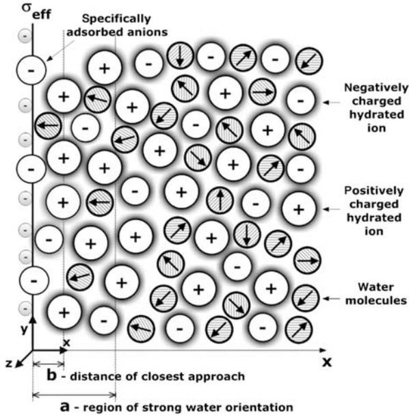
Figure 6. Charge distribution SLB model (Gongadze et al. 2011c), where in the interval  $0 < x < a$  is the region of strong water orientation and  $b$  is the distance of closest approach. The surface charge density  $\sigma = \sigma_{\text{eff}}$  incorporates the negatively charged metallic surface, as well as the specifically bound negatively charged ions (Butt et al. 2003).
