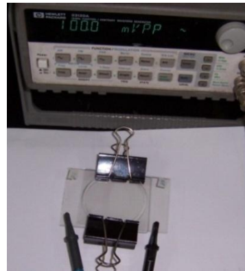
Figure 3 (b). An image of the electroformation set-up (electroformation cell connected to the generator).
